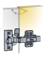
Slightly open the door to hear the click meaning angle restrictor is in the right position
