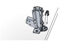
Insert angle restrictor into the hinge cup
