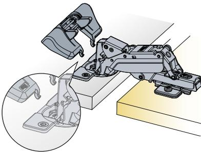
Insert Glissando TL 170 into the holes on the hinge cup
