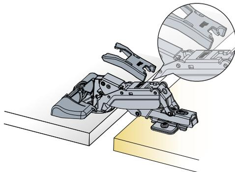
Place the striking plate into the hole on the hinge arm
