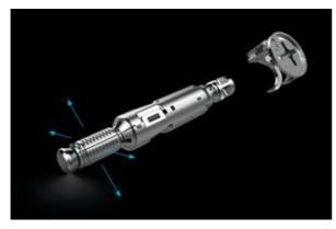
Quickfit 'Full Metal Jacket' is a highperformance Quickfit connector family with greater resistance to dowel pullout, providing optimal strength and effective performance in multiple wood-based materials, including MDF, chipboard and solid wood. Quickfit TL5 dowel is developed to make cabinet assembly fast and easy with tool-free insertion. Its unique expandable metal sleeve is the main feature that provides reliable
