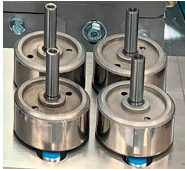
The 371 type rotors are part of the electric motors used for mowers and other electric hand tools in Husqvarna
