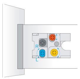
Slimline+ features a **colour-coded adjustment panel** positioned at the front, providing easy and intuitive access for quick and accurate finetuning. The panel incorporates a **three-dimensional front adjustment mechanism**, ensuring precise alignment and enhanced user convenience.
