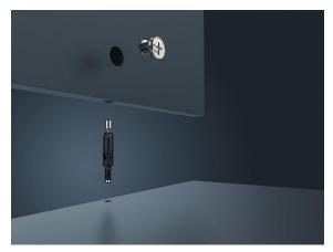
Quickfit TL5 dowel, an award-winning solution, is the fastest fitting on the market, developed to make cabinet assembly fast and easy with tool-free insertion. Thanks to its unique expandable steel sleeve, it is the only dowel on the market that reliably engages in a 5mm dowel hole, enabling the use of the tool-less Quickfit dowel insertion technology across a wide range of applications in RTA furniture where 5mm drilling is the standard, thus maintaining rigid furniture construction
