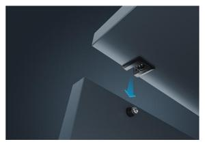
The new System 6 square design is not only modern and elegant, but also allows a larger surface of the product to rest on the panel when tightened to achieve optimal position parallel to the board surface. There is a better coverage of the drilling hole preventing possible panel damage made at drilling.
