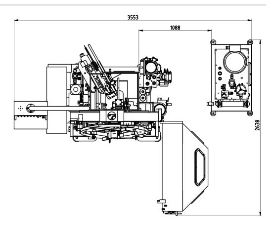
The H100 machine is a compact machine with a small footprint. To the rear of the machine there should be a minimum clearance of one metre to allow for access to the melt pot, injection unit. Space should allow for any lifting equipment and personnel access needed to carry out machine operation and maintenance tasks on and around the machine.
