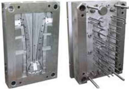
Tools for production of parts from thermoplastics.
