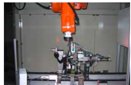
Pedal box robot video inspection
