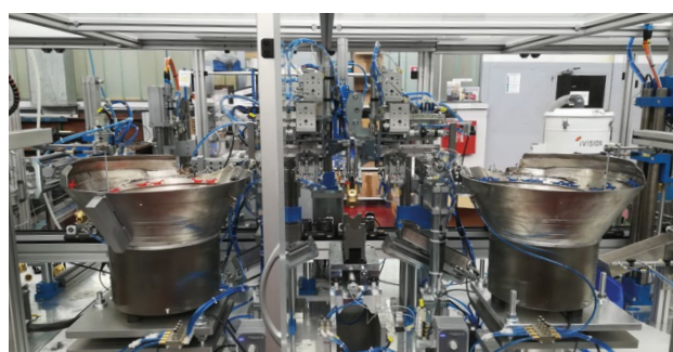
Assembly taking place on the pallets of the transport system and on rotating distribution table.
