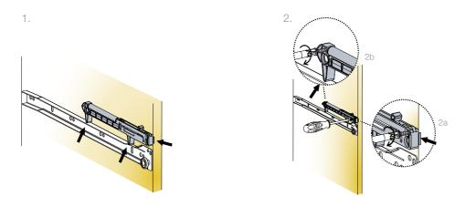
Position the Titusoft mechanism on the top of the drawer slide
