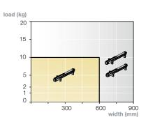
Mount 1 or 2 Titusoft mechanisms depending on drawer weight and width
