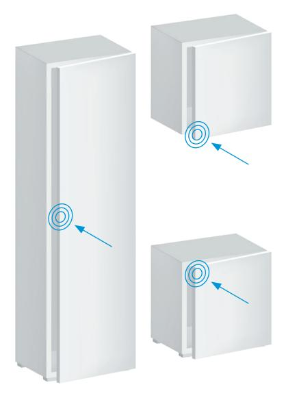
For optimal performance, the mechanism should be positioned near the 'touch opening point' on the cabinet side opposite the hinges.
